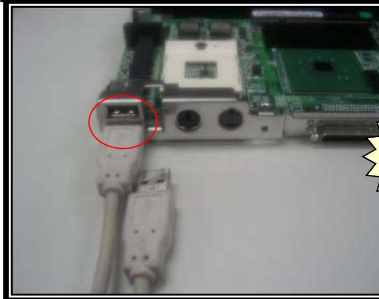
**Plug USB TEST Fixture into USB connector(RJ-45).**
