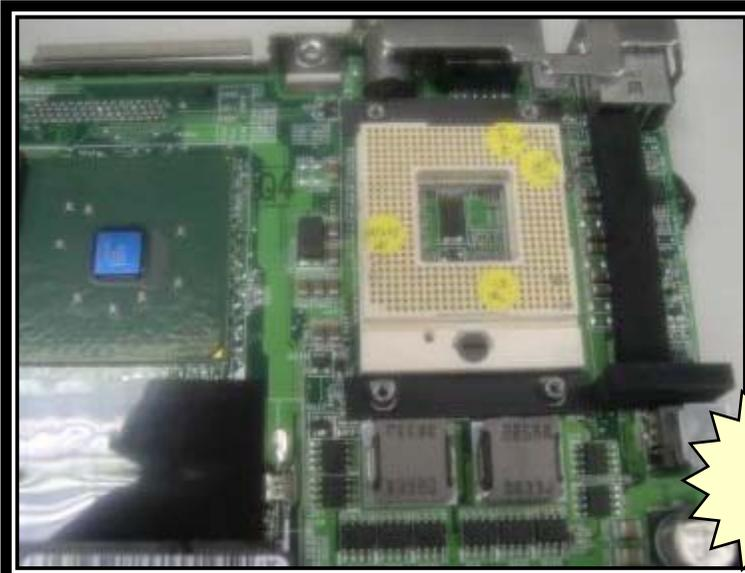
**1.Plug CPU Voltage tool into CPU socket**
