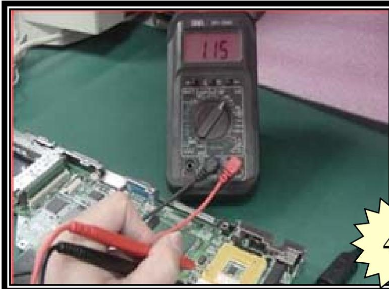
**Use Multi-Meter or Oscilloscope to Measure CPU Voltage (VCORE) on CPU Voltage tool (+10% voltage to permit)**
