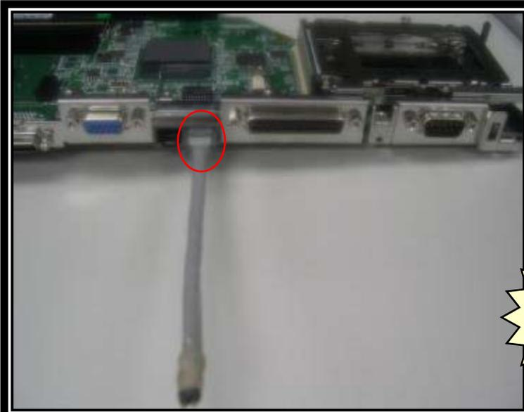
**Plug LAN loop back TEST Fixture into LAN connector(RJ-45).**
