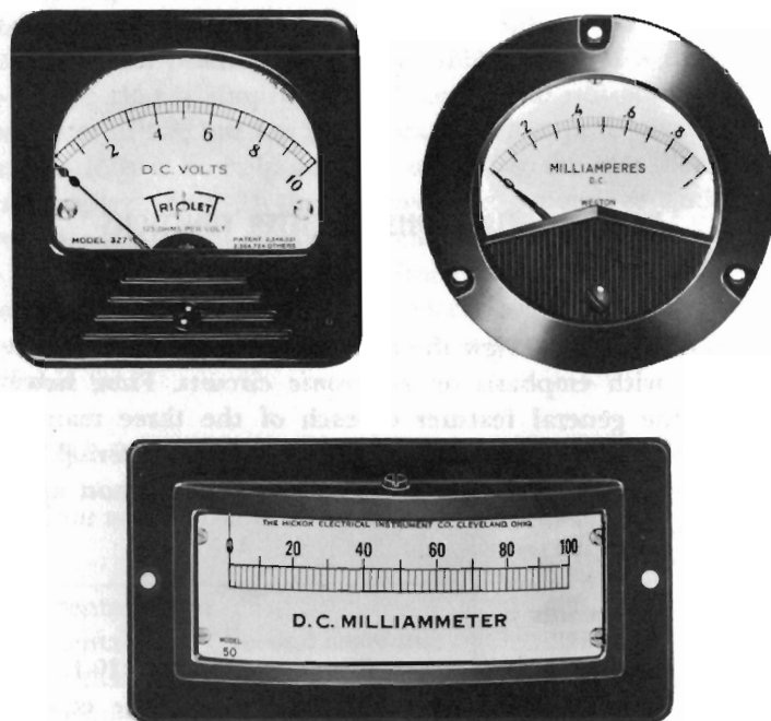
Fig. 10-1. Photographs of typical, modern panel meters. (Note: The above photos are reproduced through the courtesy of the manufacturers indicated.)
